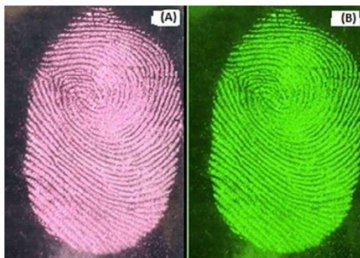
Fig. 2: Fingerprints developed on glass using ST-R (A) under White light, (B) under Fluorescent light
